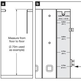
**10.** Measure the distance between the floor of the room to the floor of the loft (2.70m used as example) (**a**). Place paper template (**G**) on back ladder section with the cutout lining up with the top hole. Position the stop at the required height (2.70m used as example), tighten both stop screws (**b**). Repeat with stop on other side of ladder.
