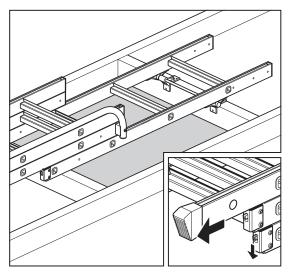
**12.** Using a suitable ladder gain access to the loft and position the ladder centrally across the loft opening with the pivot assembly resting squarely on the trapdoor surround. To help with access, release the locking catch on the end of the top ladder section and slide the middle and bottom sections down the ladder.
