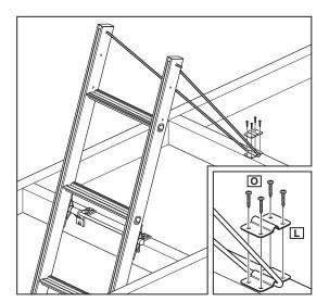
**16.** Attach the pivot arm to the loft floor/wooden batten (this may have to be added at the correct distance) using the pivot arm bracket. Use a bradawl or small drill to start the screw holes, attach the bracket (L) to the loft floor using 4 x 20mm screws (**O**).
