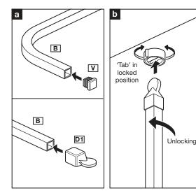
**5.** Fit the ends to the pole (**a**). **To lock:** Turn anticlockwise, **To unlock:** Turn clockwise (**b**).
