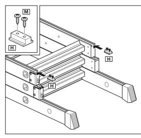
7. Loosely insert 12mm screws  $({\rm M})$  into both stops  $({\rm H})$  and slide into the top ladder section.
