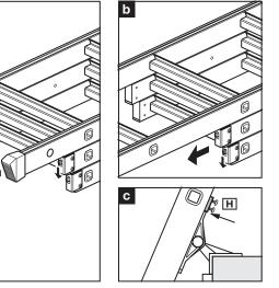
**14.** From below, fully extend ladder out of loft opening. Release the locking catch from below on middle ladder section and extend bottom section until it locks (**A**). Repeat with the catch on the top section and extend the middle section until it locks (**B**) **Important:** Ensure top stops (**H**) are tight against glides (**C**) and feet sit evenly on the floor below.
