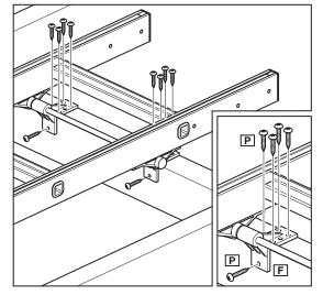
**13.** Ensure both pivots (**F**) are spaced as far apart as possible (up against the glides). Use a bradawl or small drill to start the screw holes, attach the pivots to the trapdoor surround using 10 x 25mm screws (**P**). Note: The trapdoor surround must be solid wood. Chipboard or composite board will not be strong enough.
