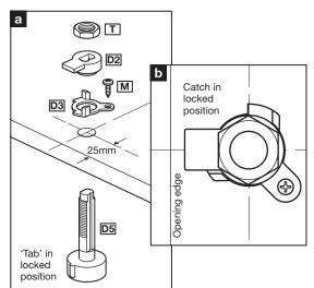
**3.** Assemble the catch. Assemble the catch onto the trapdoor ensuring the 'tab' on the catch barrel and the catch are positioned as shown (a). Note: Only fix the retaining washer (D3) using the 12mm screw (M) once correctly positioned as shown above (b).
