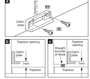
**4.** Attach catch plate. Find and mark the centre line onto the opening end of the trapdoor surround. Allow a 7mm gap between the top of the catch plate and the trapdoor (**b** or **c**). Attach the catch plate (**D4**) to the trapdoor surround using  $2 \times 12$ mm screws (**a**).
