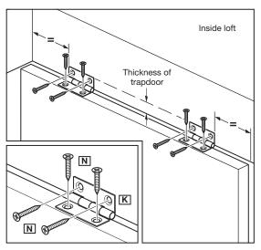
**1.** Attach hinges to trapdoor and opening. Drill 2mm pilot holes, attach hinges (**K**) to trapdoor and surround using 8 x csk 20mm screws (**N**). Note: The trapdoor will attach to the same side of the opening as the ladder (Trapdoor is not supplied).
