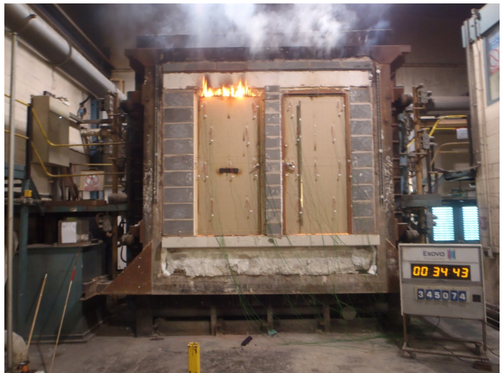
The unexposed face of the doorsets after 34 minutes of testing as sustained flaming formed at the head of Doorset A
