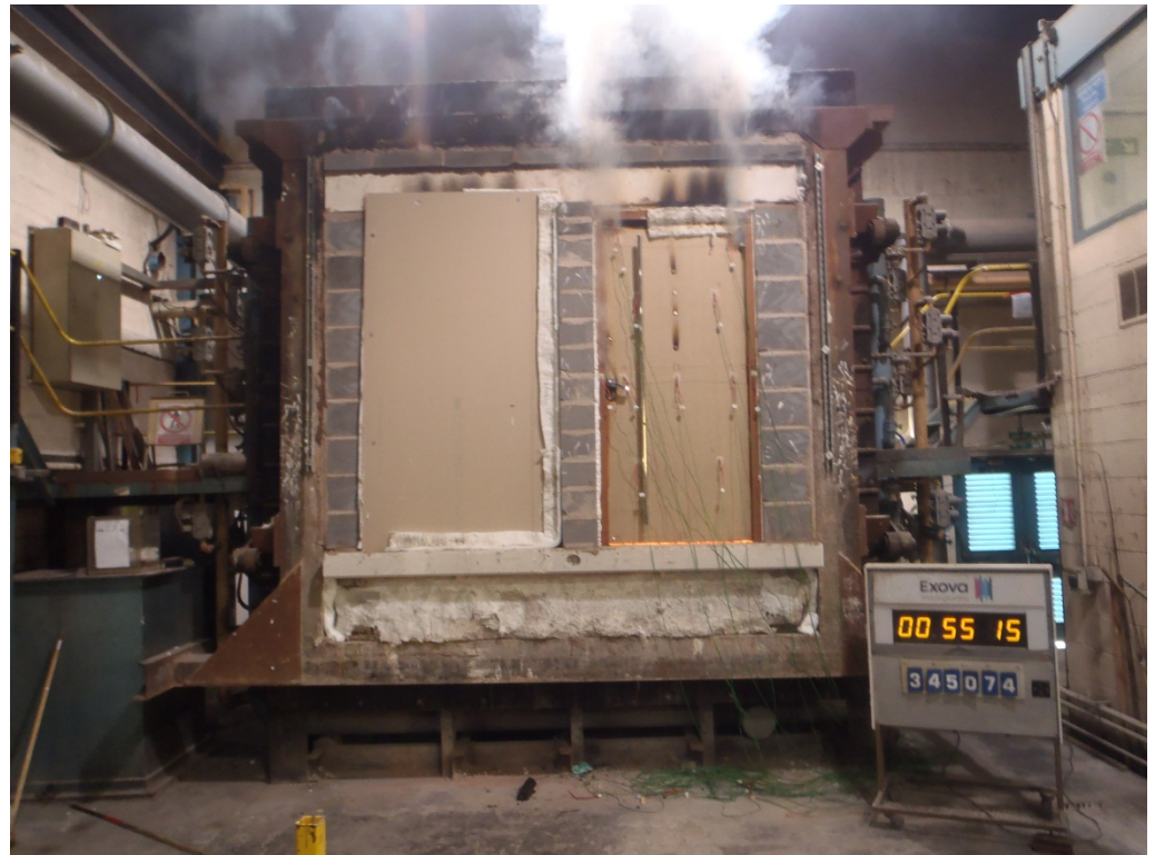
The unexposed face of the doorsets after 55 minutes of testing
