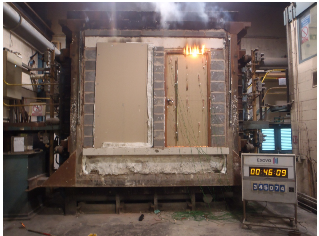
The unexposed face of the doorsets after 46 minutes of testing as sustained flaming formed at the head of Doorset B
